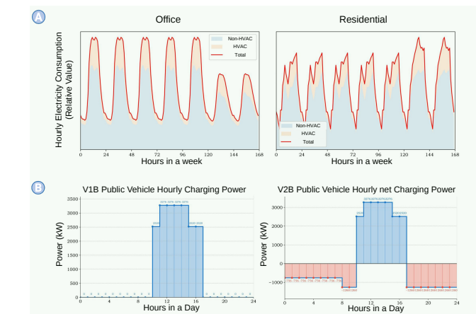
Figure 6. Surrounding Resource Settings (a) Load profiles of surrounding buildings. (b) Net Charge Load profiles of Public Vehicles.
