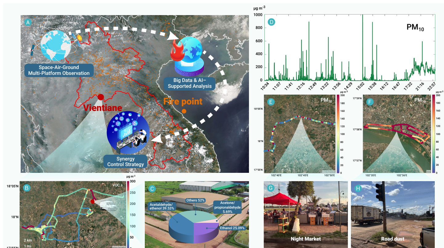
Figure 1. Conceptual diagram of the China-Laos air quality initiative and preliminary observational findings (A) Spatial distribution of fire hotspots in Southeast Asia during the 2024 dry season. (B) Mobile monitoring route and VOCs concentration distribution. (C) Aerial view of an industrial park and detected VOCs species. (D) Temporal variations in PM 10 concentrations. (E-F) Spatial distribution of PM 10 in typical source areas. (G-H) Field photographs of typical pollution sources.
