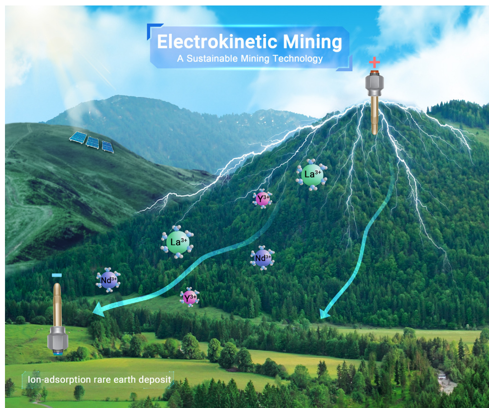
Figure 1. Illustration of IAD mining via EKM The hydrated REEs are expected to be mobilized, transported, and extracted from an IAD under an applied electric field.
