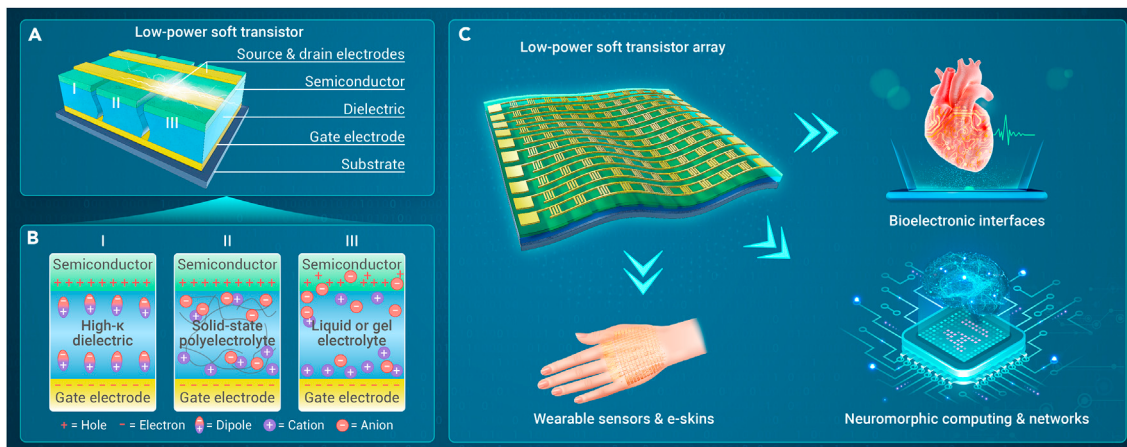
Figure 1. Comprehensive overview of low-power soft transistors (A) Schematic diagram of the device structure. (B) Illustration of the working principles based on three types of dielectric materials. (C) Promising prospects for applications in emerging electronics.
