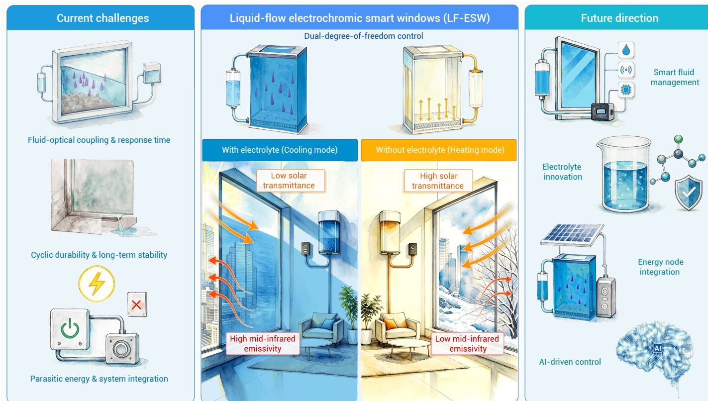
Figure 1. Overview of challenges and future directions for liquid-flow electrochromic windows.
