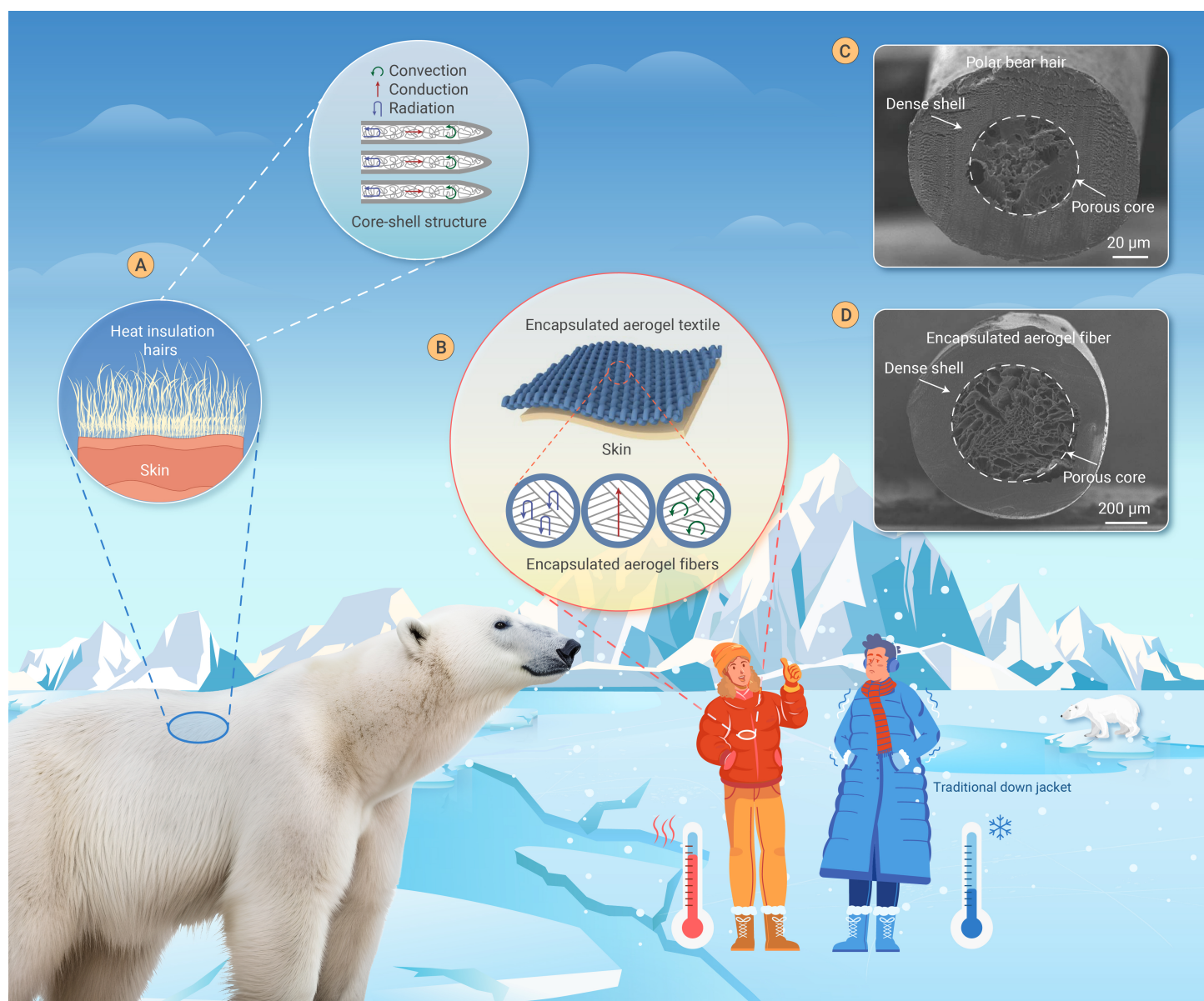
Figure 1. Biomimetic encapsulated aerogel fibers (A) Schematic diagram of thermal insulation principle of polar bear hair. (B) Schematic diagram of thermal insulation principle of EAFs and comparison of corresponding fabric property with traditional down jacket. (C-D) SEM images of polar bear hair and EAFs. 5 Reproduced with permission. Copyright 2023, American Association for the Advancement of Science.
