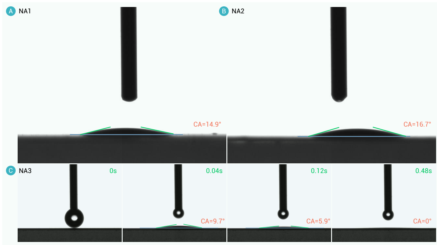
Figure 5. Contact angle measurements (A) static contact angle for the sample NA1, (B) static contact angle for the sample NA2, (C) the dynamic contact angles for the sample NA3.
