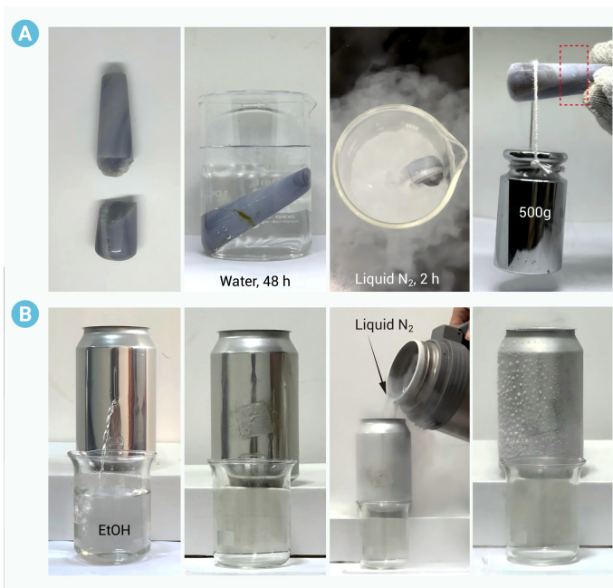
Figure 7. Illustrations of various applications of P(C_{0.4}\text{-}co\text{-}G_{0.6}) adhesive (A) The fractured agate mortar pestle can be repaired and guaranteed its performance after immersing in water and liquid N_2 . (B) The leakage of a barrel holding a solvent ( H_2O and EtOH) can be rapidly repaired using a foil paper coated with slightly heated P(C_{0.4}\text{-}co\text{-}G_{0.6}) adhesive.
