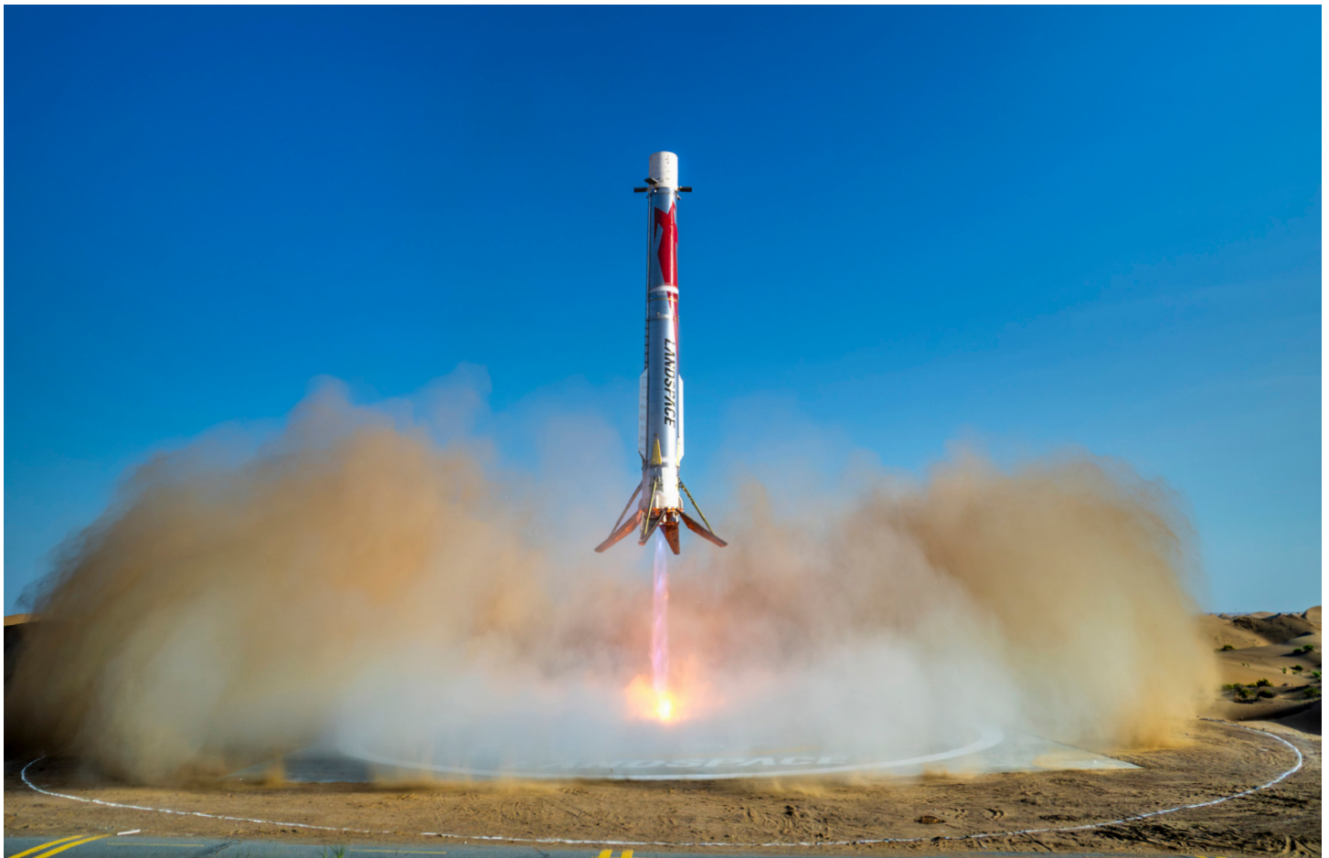
Figure 1. Zhuque-3 Y2 first-stage successful landing recovery Officially authorized by LandSpace
